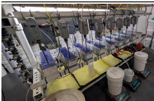
Figure 49: Once leachate is recovered, it's processed through a conventional solvent extraction circuit...
